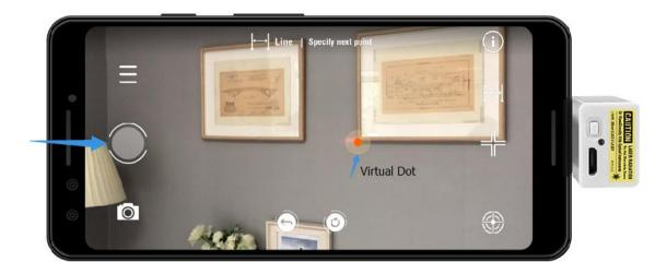
Aim the laser dot to the end of the line, and tap Measure button again, another virtual dot will be placed, and the measurement result will be shown.
