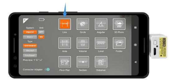
Aim the laser dot to the start of the line, and tap Measure button. A virtual dot will be placed there.
