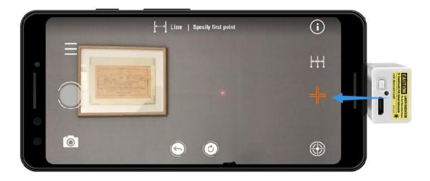
In this mode, you aim the laser dot to **Point A** and tap the <u>Measure</u> button. A plane and vertical line appears, and You aim the laser dot to edge of wall, and the software will automatically find the perfect horizontal **point B** on the edge and provide you the measurement of D. It works for vertical situation as well.
