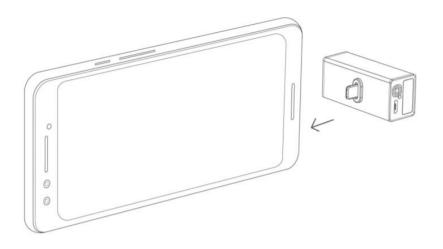
• Insert Arrim ONE to the mobile device. Laser is facing out.
