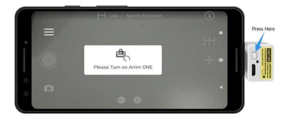
• Arrim ONE will be connected automatically with the mobile device via Bluetooth. The laser will be on, and you can see a bright red laser dot.
