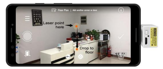
Specify the corners one by one. And tap the **<u>Door</u>** button for door frame begins, and tap the **<u>Door</u>** button again for door frame ends. The virtual points for doors are blue.
