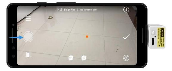
Point the laser to first corner and tap <u>Measure</u> button. If there is obstacle, you can move up the Laser beam, and tap <u>Measure</u>, the point will automatically drop down to the floor.
